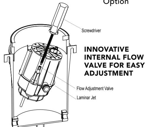
INNOVATIVE INTERNAL FLOW VALVE FOR EASY ADJUSTMENT
